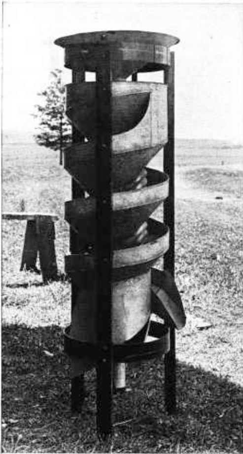
Figure 8.—A spiral vetch separator, an efficient separator for removing rye or other small grain from vetch.
